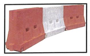
When water barricades are filled and connected pursuant to the manufacturer's instructions, the barricades will deflect a vehicle traveling at 45 mph. Using additional signs and Type III barricades alone will not prevent an errant vehicle from entering a pedestrian zone; however, rigid barriers provide the segregation of pedestrian and vehicular traffic required to meet pedestrian safety measures.
