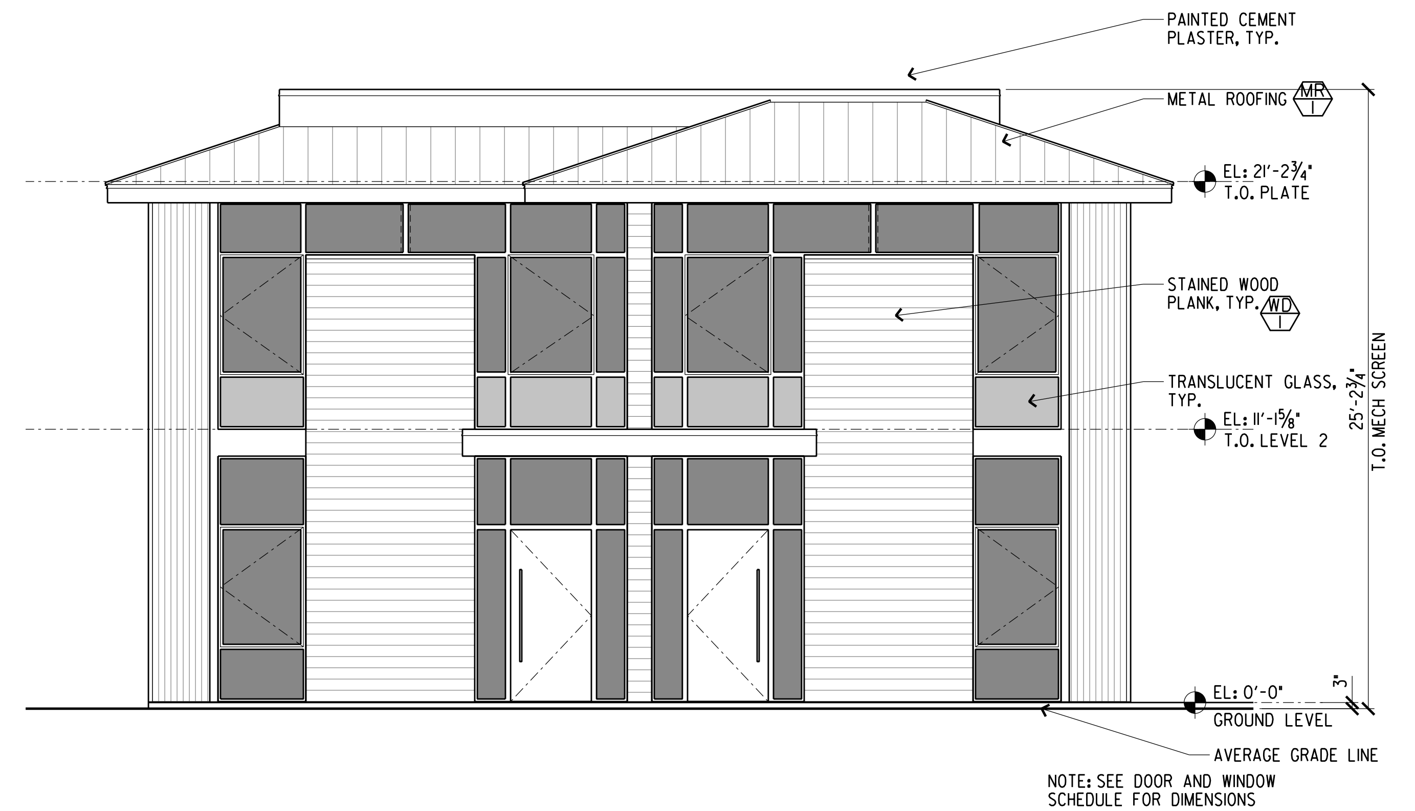
B1 SCALE: 1/4"=1'-0" NORTH ELEVATION - NORTH BUILDING
