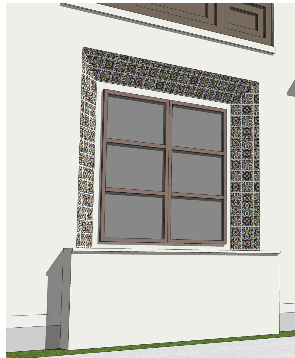
18/23 ACCENT BATTERED CERAMIC TILE SURROUND w/ TILE CAPPED BARRANCA
