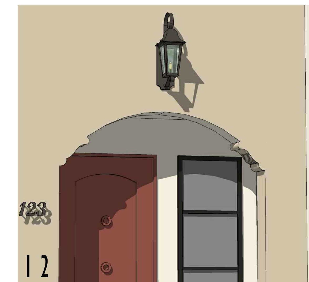
12 STUCCO ARCH w/ CORBELS
