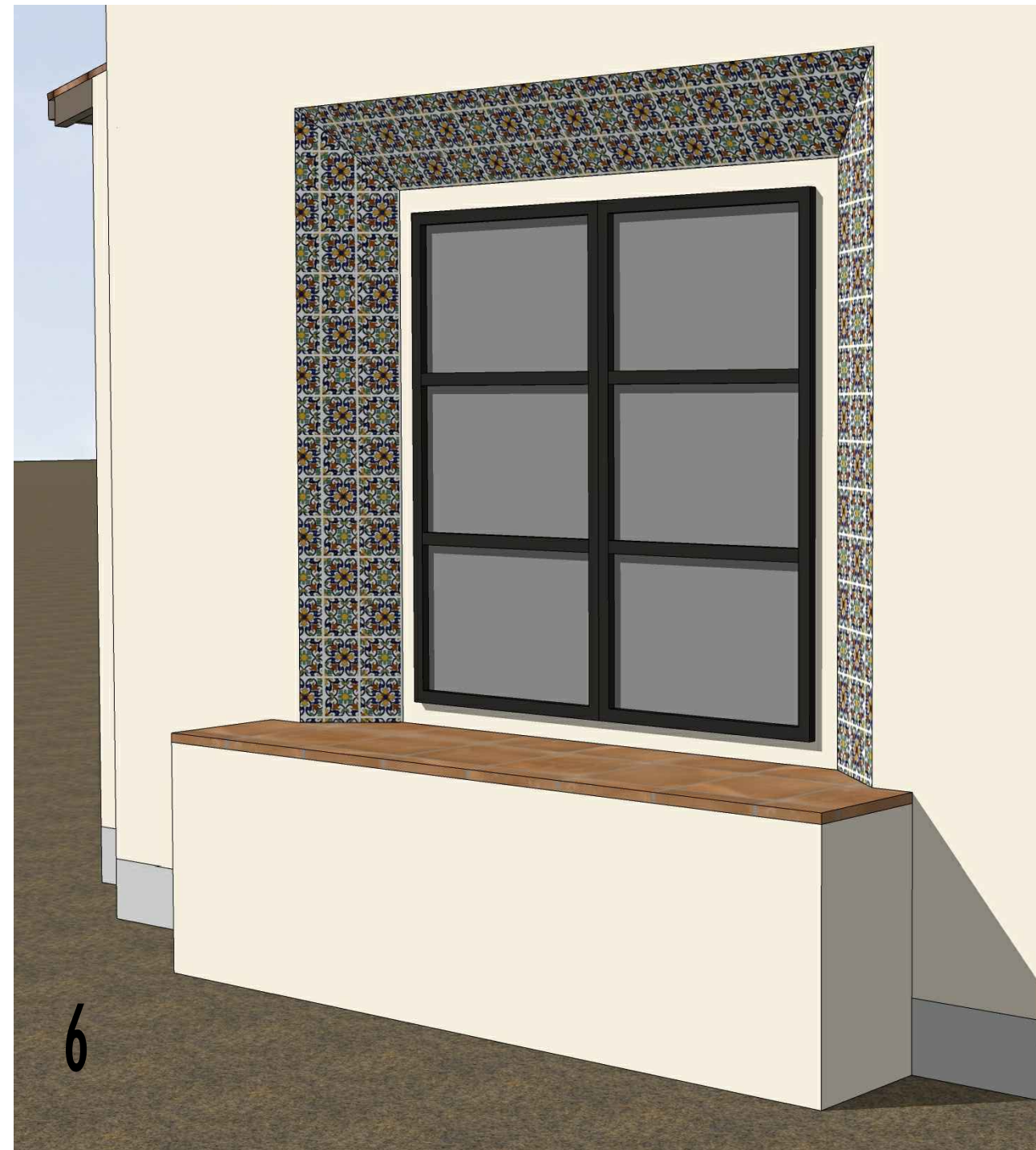
6 ACCENT BATTERED CERAMIC TILE SURROUND w/ TILE CAPPED BARRANCA
