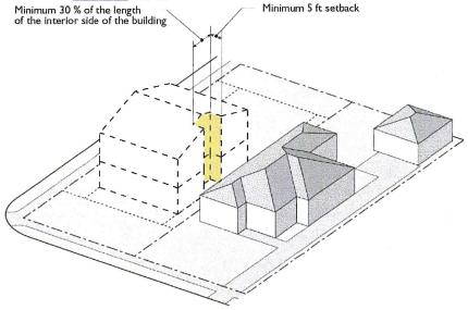
c. Standard E-(2)( $\subseteq$ c): The second story setback is determined by a 45-degree inclined daylight plane extending from the intersection of the side property line and the existing grade at a point 12 feet above finished grade. See Diagram 10.1.603(E)(2)(C) below.
