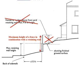
e. Additional retaining walls must be setback a distance equivalent to twice the height of the exposed retaining wall below as measured from the face of the retaining wall below lowest abutting finished ground surface, after any grading, cut, or fill activity.
