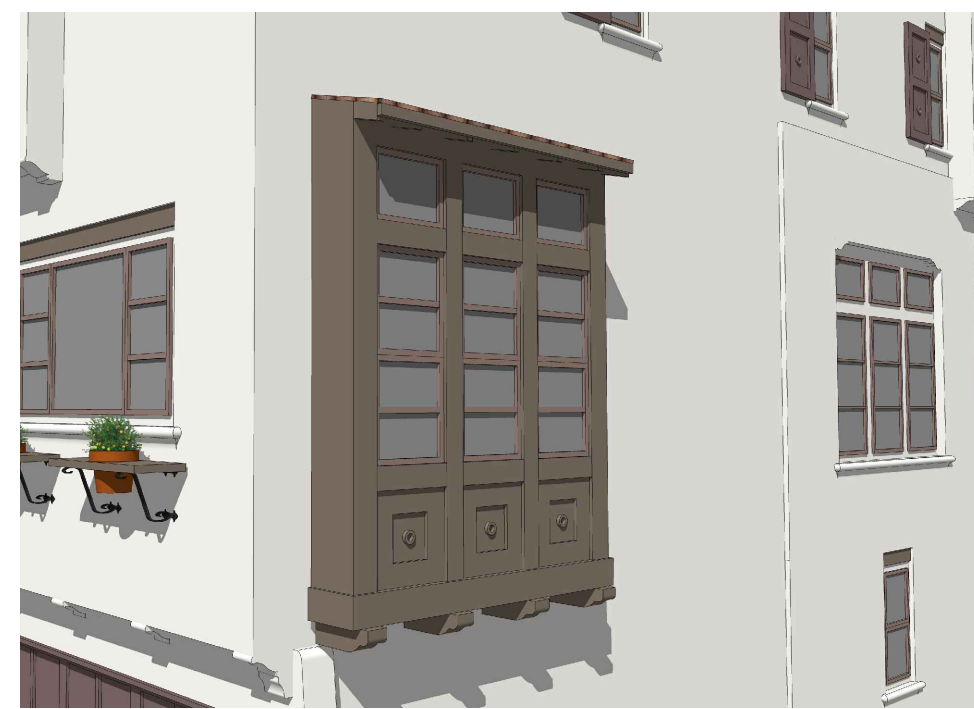
9 BOX BAY WINDOW w/ FIBER CEMENT BOARD PANEL, FAUX WOOD CORBELS
