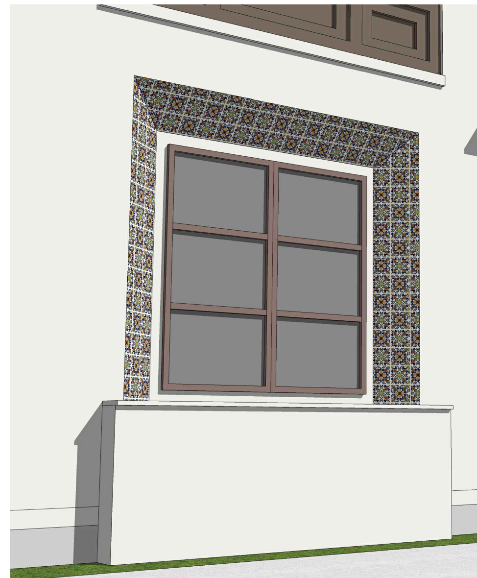
7 ACCENT BATTERED CERAMIC TILE SURROUND w/ TILE CAPPED BARRANCA
