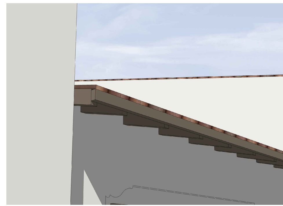
3 TYPICAL EXPOSED WOOD TRUSS TAILS
