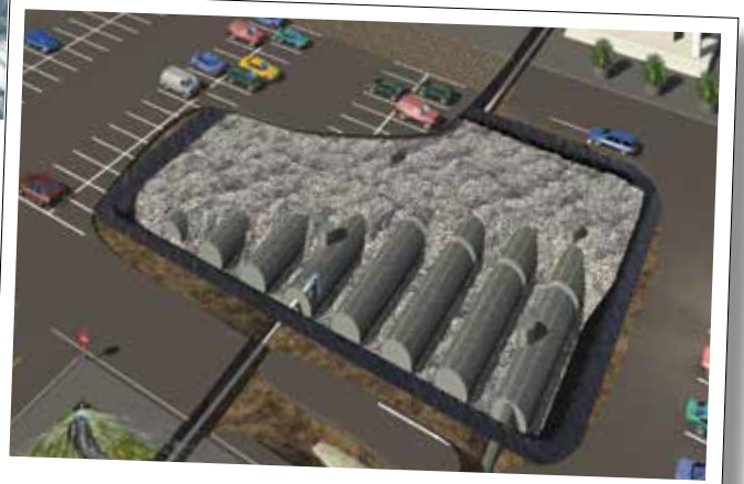
Stormwater runoff is stored in the pipe and surrounding stone
