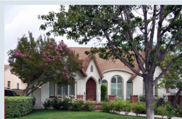
Figure 28 - The rolled eaves, steep roof, vertically proportioned windows and doors, and Gothic style arch of the entry door are indicators of a Storybook style home.
