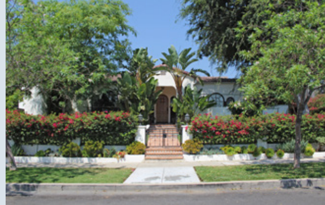
Figure 48 - Fences, walls, and hedges, if provided at front yards, need to meet City height requirements and should be set back from the back of sidewalk to provide landscape opportunities on both sides.
