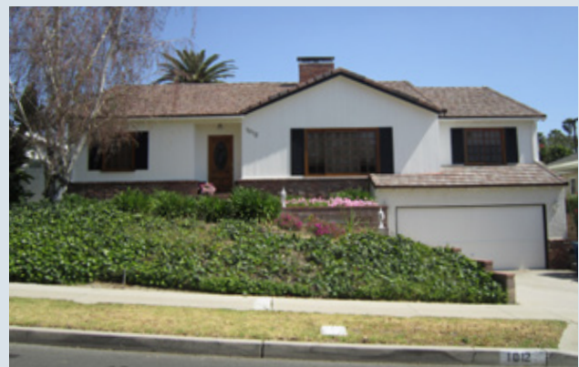
Figure 11 - Changes in topography across Cut Hillside lots often allows garages to be discretely tucked into the cross-section of a parcel.
