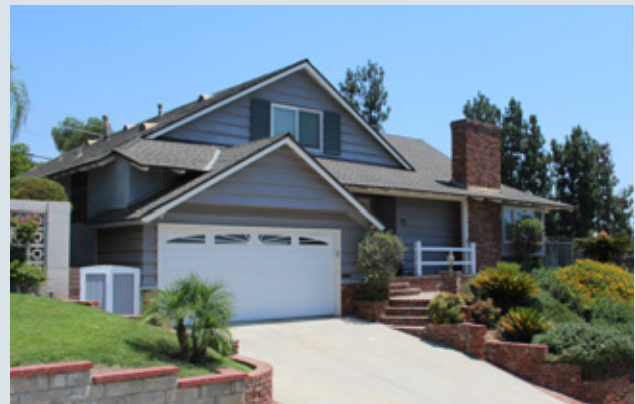
Figure 38 - The overall bulk of this home is reduced through the introduction of two smaller masses, the gabled second-story mass that is smaller than the overall bulk, and the subordinate garage mass. The chimney creates additional variety and interest and a sense of smaller scale.
