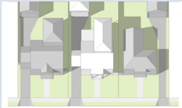
Figure 35 - In those locations where garages are typically placed behind the home, this built-form pattern should be respected.
