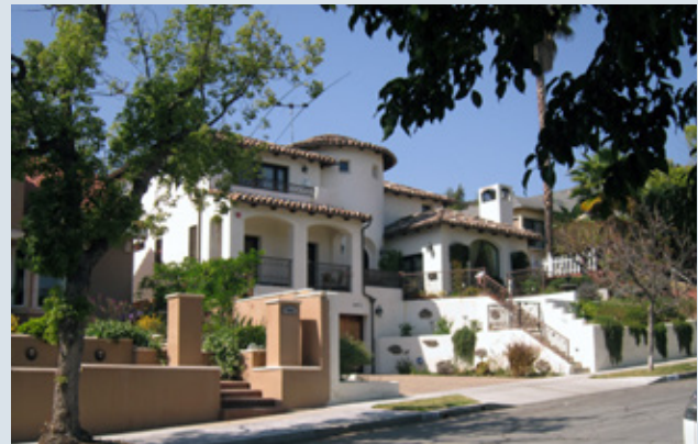
Figure 37 - The tower element breaks the line of the roof ridge. The three smaller masses contrast with the overall bulk, reducing the perception of a large, box-like form.
