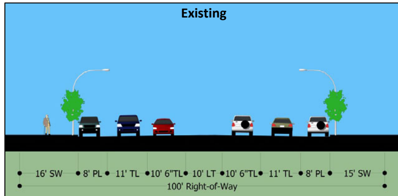
Figure 4-1b: North San Fernando Boulevard: Typical Section from Andover Drive to Scott Road (Looking Northwest)
