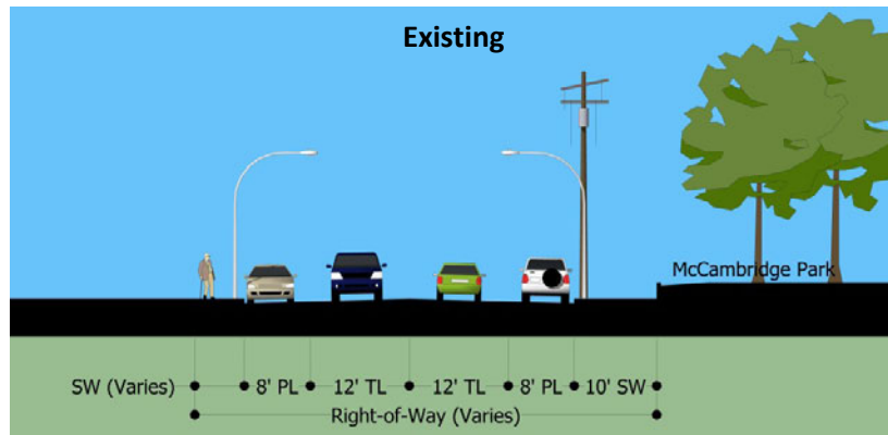
Figure 4-3b: Scott Road: Typical Section from East Avenue to North San Fernando Boulevard (Looking Northwest)
