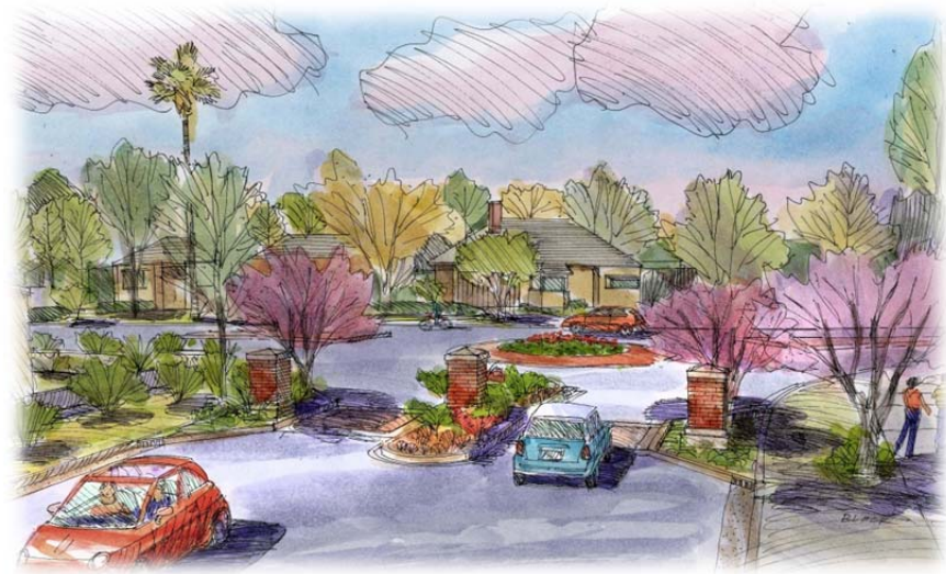
Conceptual view of lane chokers, island planter, neighborhood entry monuments and roundabout at the intersection of Amherst Drive and Broadway.
