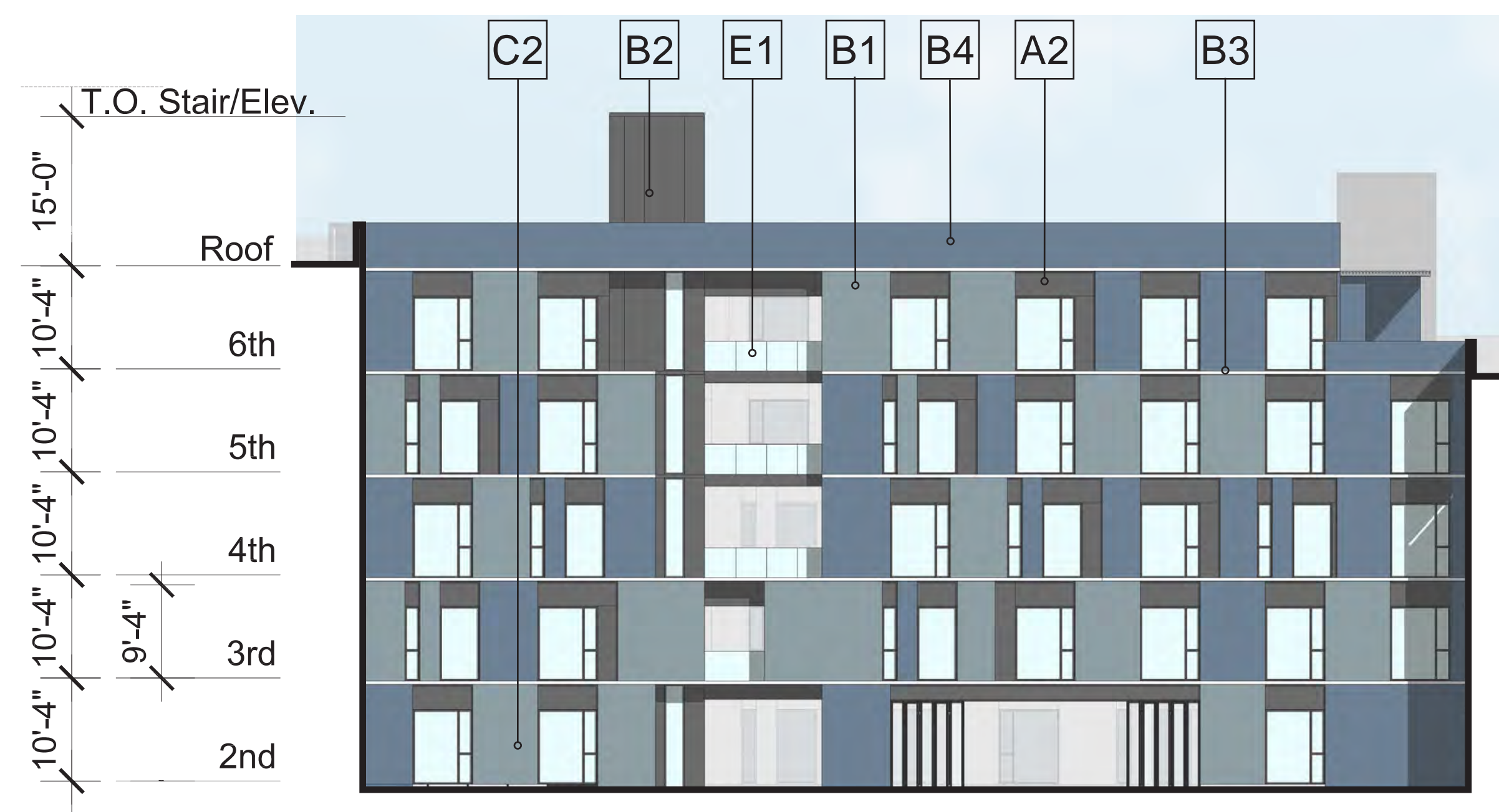
NORTH ELEVATION - COURTYARD
