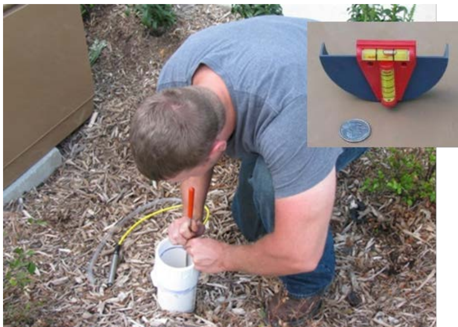
Figure 31. Typical weir for monitoring flow in an underdrain.
