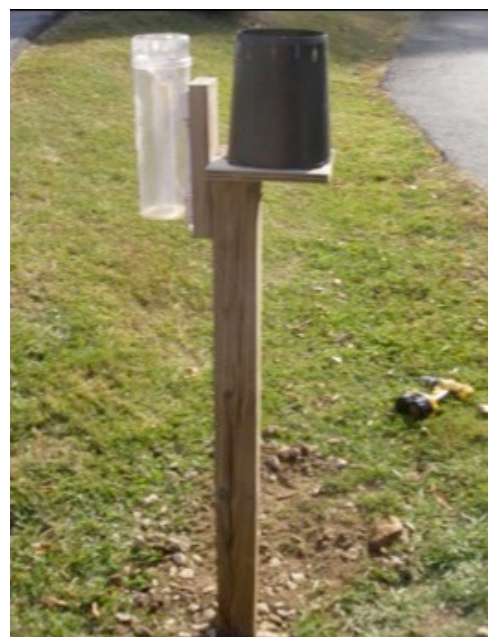
Figure 26. Example of manual (left) and tipping bucket (right) rain gauges.
