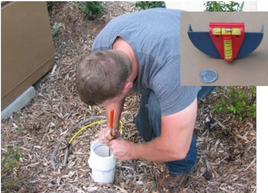
Figure 30. Typical weir for monitoring flow in an underdrain.
