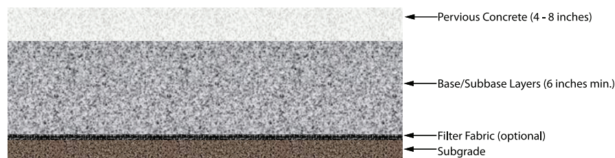
FIGURE 1. Typical pervious concrete pavement cross section (adapted from EPA 2010).
