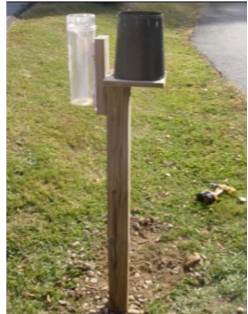
Figure 32. Example of manual (left) and tipping bucket (right) rain gauges.
