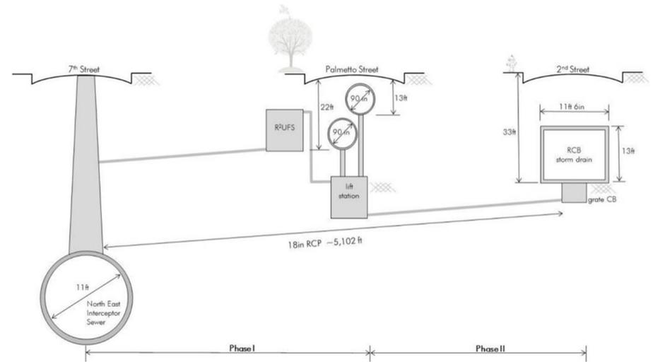
Figure 6-3. Elements of the LRS Actions for R2-02 (project is in planning phase, see Appendix E)
