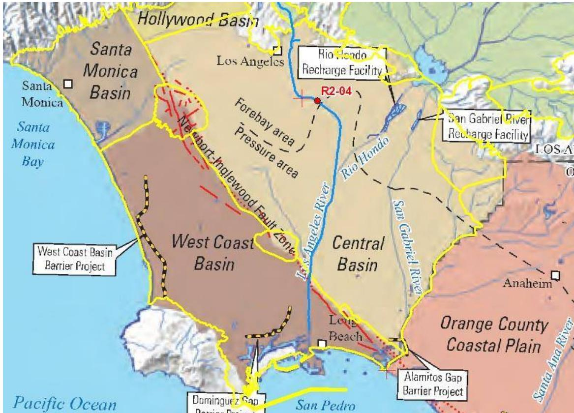
Figure 4. Georeferencing of USGS forebay and pressure area map with groundwater basin boundaries using GIS
