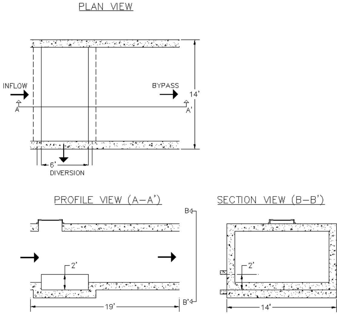
**Figure 9. Diversion structure for dry weather flows.**
