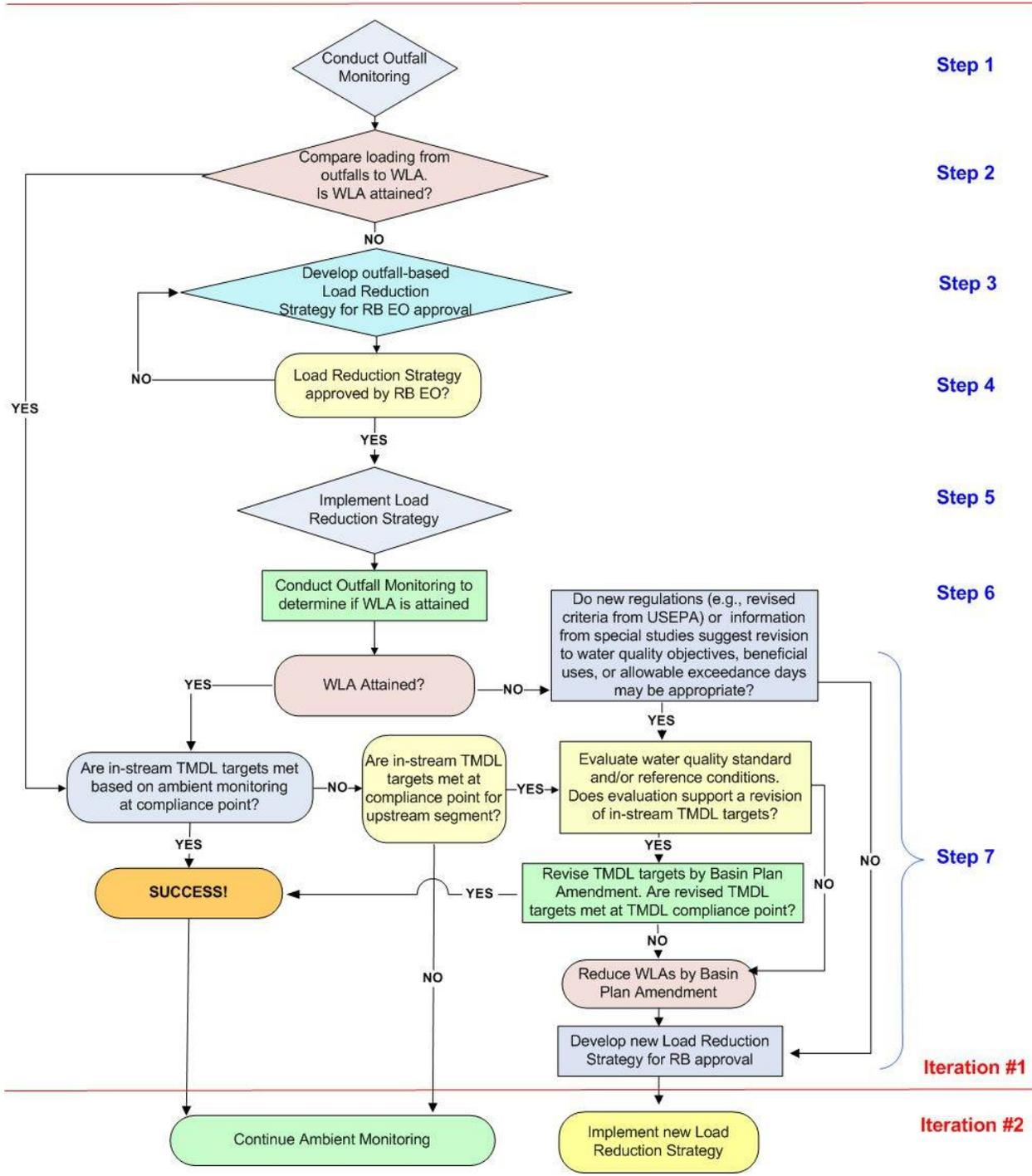
**Figure 2. LA River Bacteria TMDL Outfall-based Approach Flow Diagram**
