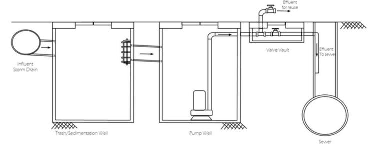
Figure 6-1. Elements of the LRS Actions for R2-A (diversion is already completed, see Appendix C)
