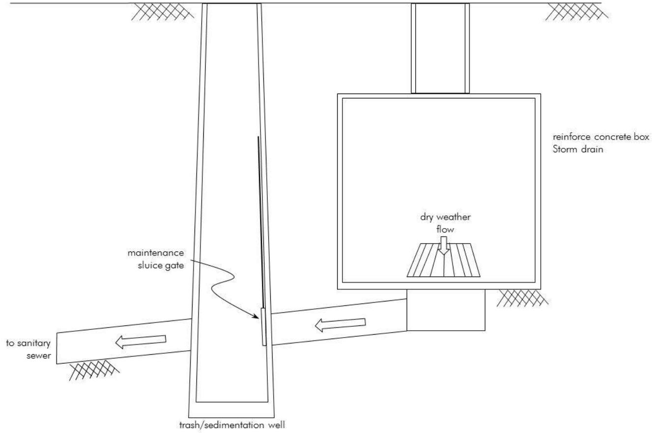
Figure 3. LFD schematic.
