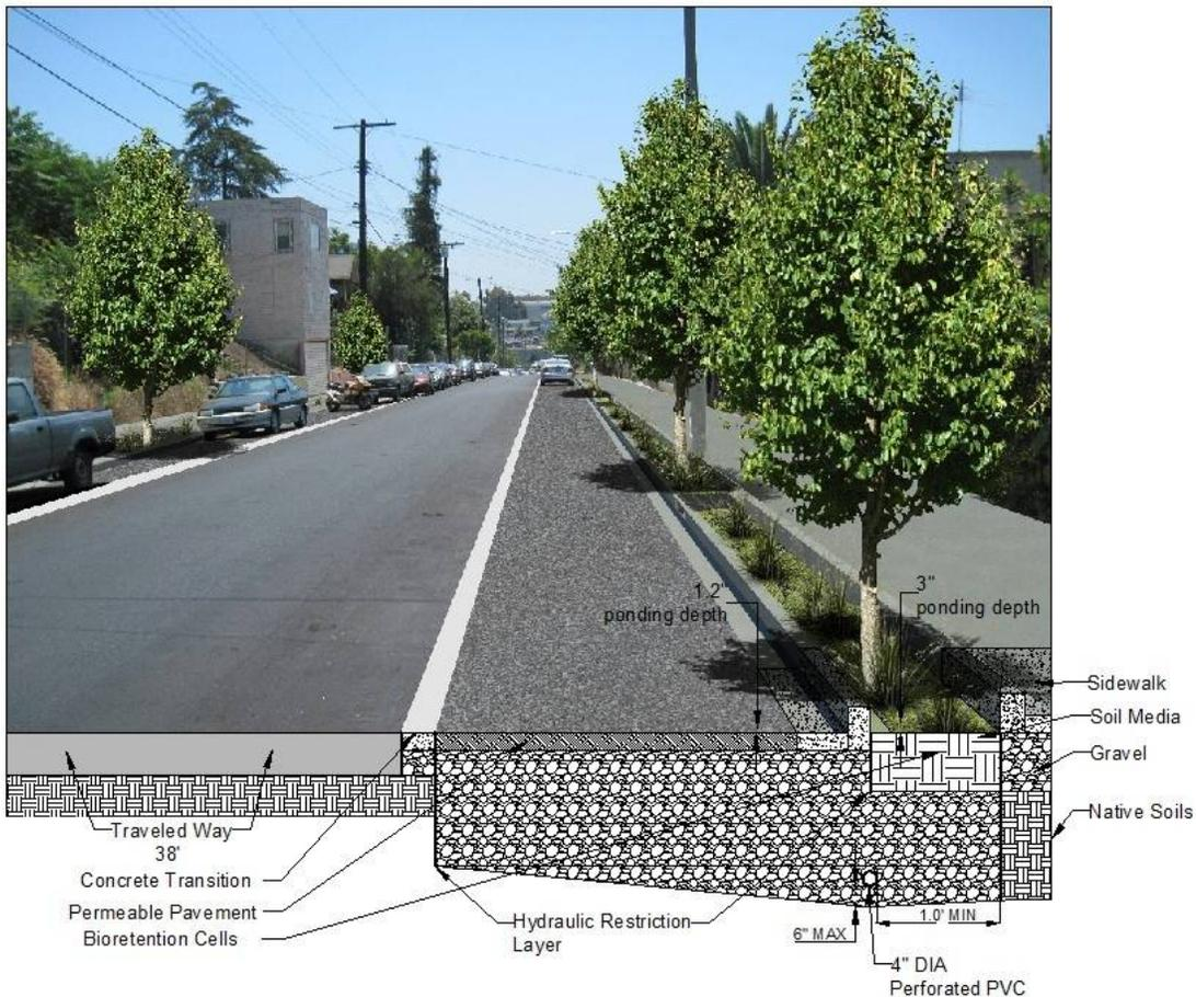
Figure 7. Greet street configuration for wet-weather treatment.
