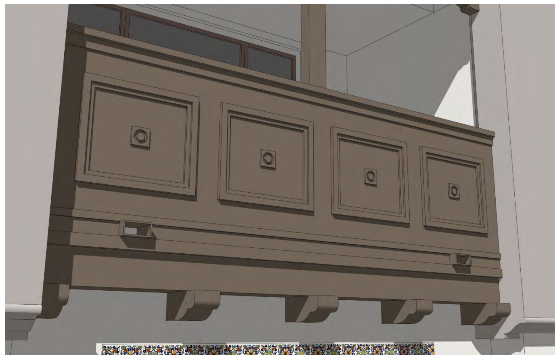
D14. Fiber Cement Railing w/ Decorative Fiber Cement Bd. Panels, Faux Wood Corbel & Deck Trim
