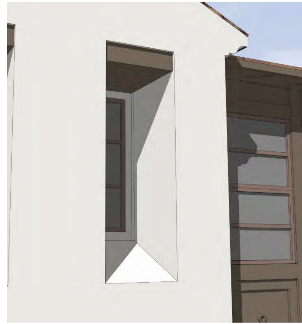
D3. Deep Recessed Window w/ 1" Recessed Stucco Simulated Wood Beam
