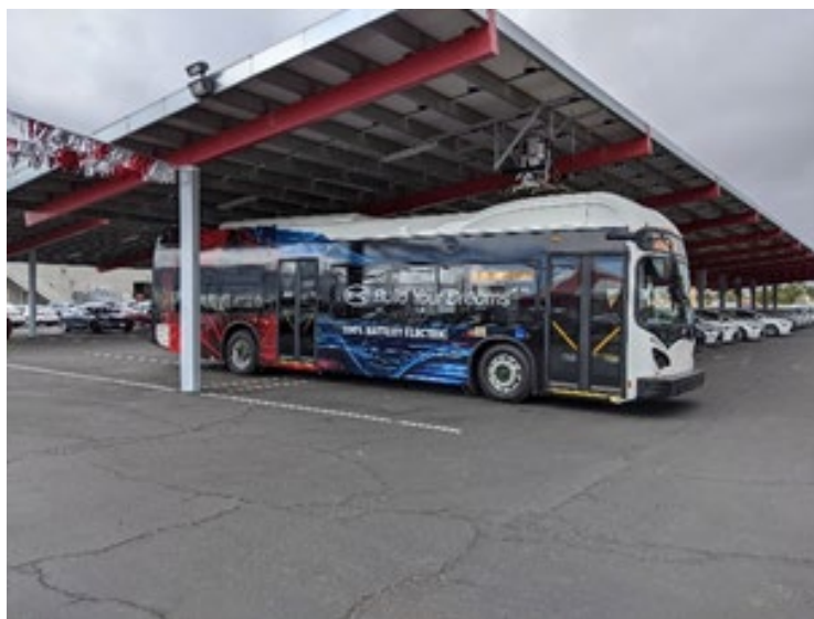
Figure 1-6: In-Depot Overhead Charging Example (Source: CALSTART)
