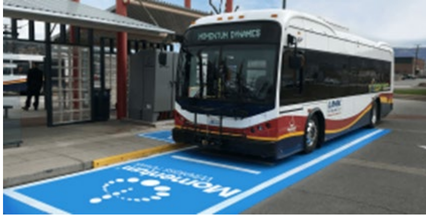
Figure 1-7: Inductive Charging Example (Source: Momentum Dynamics)
