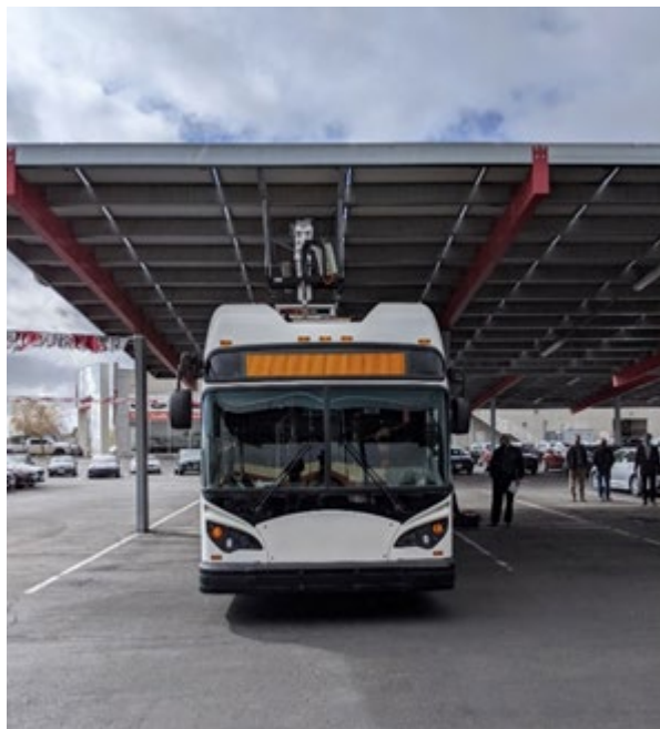
Figure 1-6: In-Depot Overhead Charging Example (Source: CALSTART)
