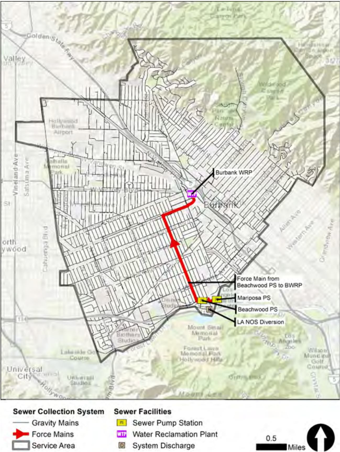
FIGURE 9-2: Burbank Sewer Collection System and Facilities
