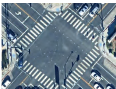
Pavement Markings Through Intersections
