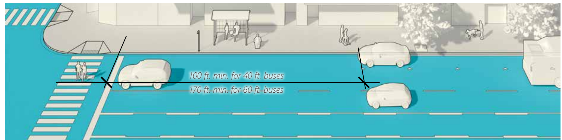
Figure 6-15. Near-Side, Pull-Out Loading Bus Stop.
