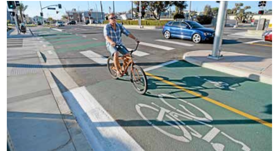
Two-Way, In-Street, Class IV Bikeway (Source: dailybreeze.com).
