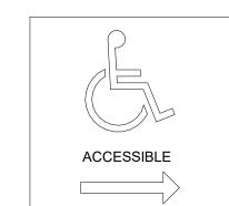
1. CHARACTER SHALL HAVE A WIDTH - TO - HEIGHT RATIO BETWEEN 3:5 AND 1:1 2. CHARACTERS SHALL HAVE A STROKE - WIDTH - TO - HEIGHT RATIO BETWEEN 1:5 TO .1:10. 3. CHARACTERS SHALL BE SIZED ACCORDING TO THE VIEWING DISTANCE FROM WHICH THEY ARE
